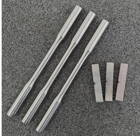
Figure 4: Machined specimens for tensile and impact tests.
