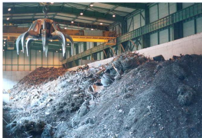
Figure 2: Scrap ready to be fed to the EAF.
